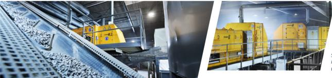
Separation of heavy from light metals with X-ray transmission technology
