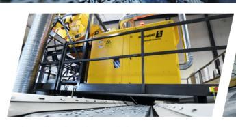
Purification of non-ferrous heavy metals down to 5 mm – into supreme copper, brass and zinc which is ready to smelt. Detected with X-ray fluorescence technology
