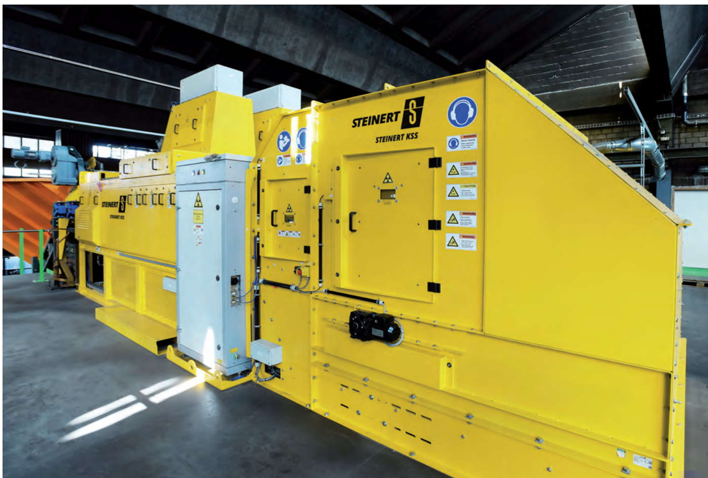
STEINERT KSS FLI XT used in ASR processing.
