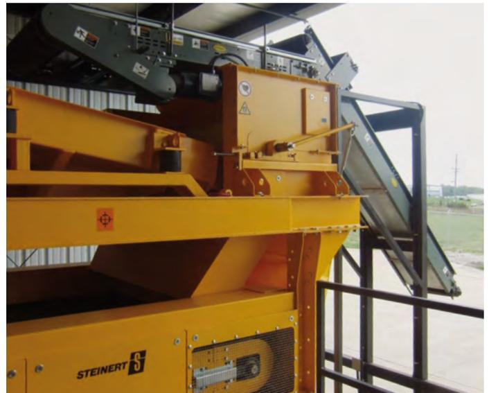
Efficient non-ferrous extraction using an eccentric pole system. Proven in operation for 25 years with more than 3,500 units sold, the eccentric pole system in the STEINERT non-ferrous separator prevents damaging iron particles from adhering and concentrates power where it is needed. The system's adjustability increases the yield by another 50%. Altogether the best possible conditions for obtaining a ready-to-sell non-ferrous product in the famous STEINERT quality.
