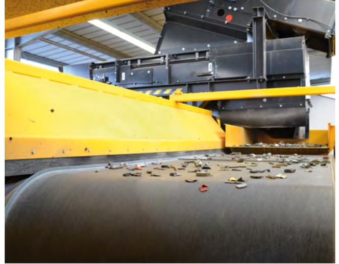
the magnetic pole system mounted eccentrically in the head drum of the STEINERT non-ferrous separators, the effect of the changing magnetic fields is concentrated exactly on an area within which the material is most effectively subject to the forces. The pole system can be adjusted so that this position can be changed in order to have the maximum effect on the discharge parabola, and so to further amplify the effect of the forces.
