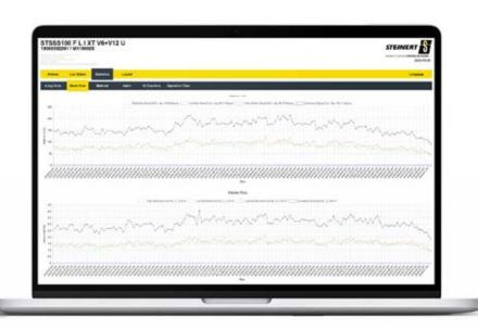
**STEINERT.dashboard** is a detailed monitoring solution for STEINERT sensor sorting systems. It enables its users to visualize operating and production figures, such as belt occupancy, volume flow, object rate, particle size distribution, active sorting program and much more, to analyze the current performance of their own sorting system and its applications.
