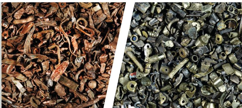
Areas of application for colour sorting are, for example, the separation of non-ferrous heavy metal concentrates in copper, brass and grey metals or the sorting of industrial minerals.
