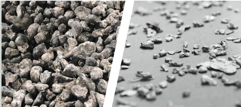
STEINERT CHUTEC sorts heavy non-ferrous metals (ZEBRA) from incineration bottom ash (IBA) or automobile shredder residues (ASR). Especially in the smaller grain sizes 05-30 mm, it ensures the separation of non-ferrous heavy metals in metal types such as copper, zinc, brass or stainless steel. The sorting system produces concentrates of different metal types, which are qualitatively suitable for the direct use at smelters.
