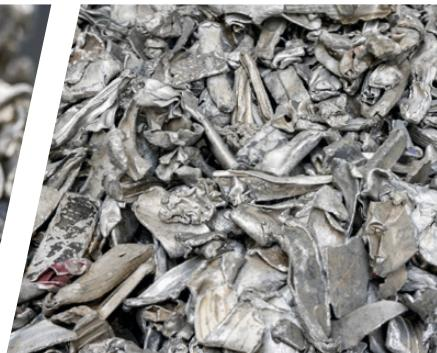
STEINERT PLASMAX | LIBS enables the efficient separation of aluminium scrap into up to three different sorted products in one pass. This solution allows recycling firms to specifically produce high-grade alloy classes ready for the furnace.
